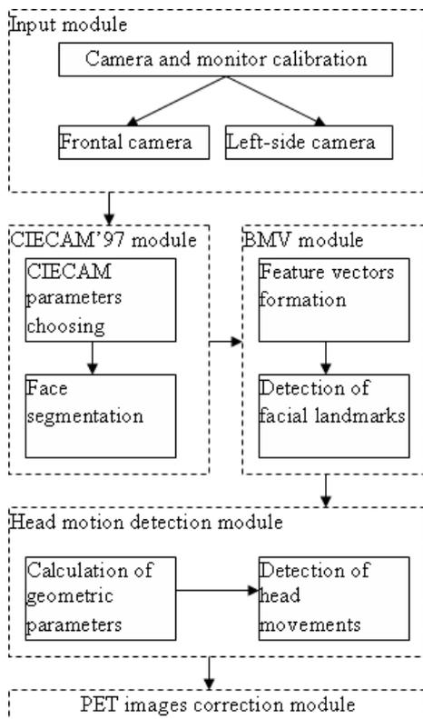
**Figure 1. The overview of the system for head motion detection.**
