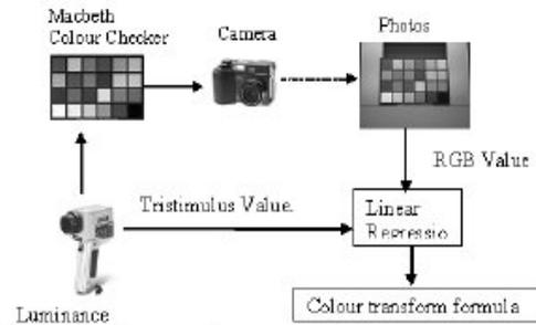
**Figure 2. The steps of camera calibration.**
