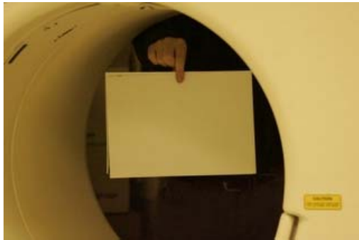
Photo shows white paper in PET scanner, this is to obtain the reference white.
